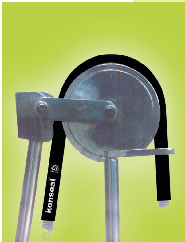
Conduit bending with the aid of spring and test apparatus.
